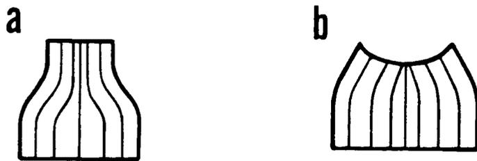
Figure A1. Schematic indication of the fiber orientation in two kinds of fiber optic taper. (a) Standard magnifier/condenser: fibers perpendicular to two flat surfaces. (b) Fiber optic taper used for these studies. Note how fibers are approximately normal to curved surface.
